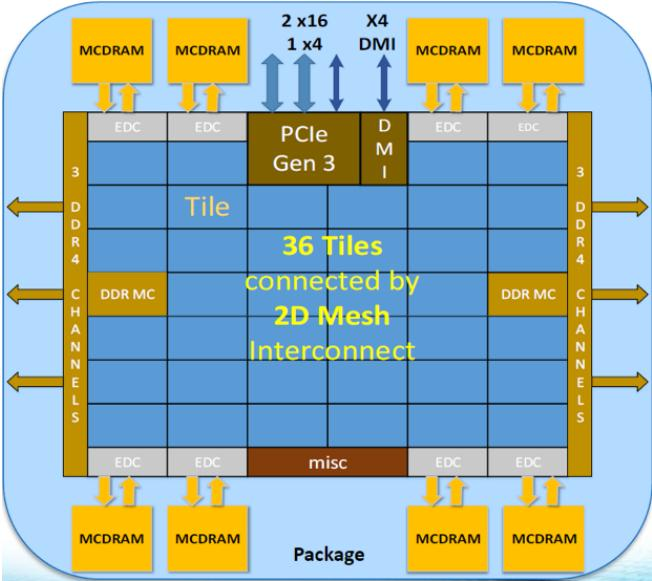
Fig. 1. KNL Processor (Credit Intel)
