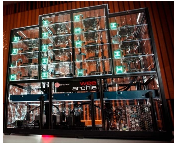
Figure 1. Wee ARCHIE: LED lights display node activity
