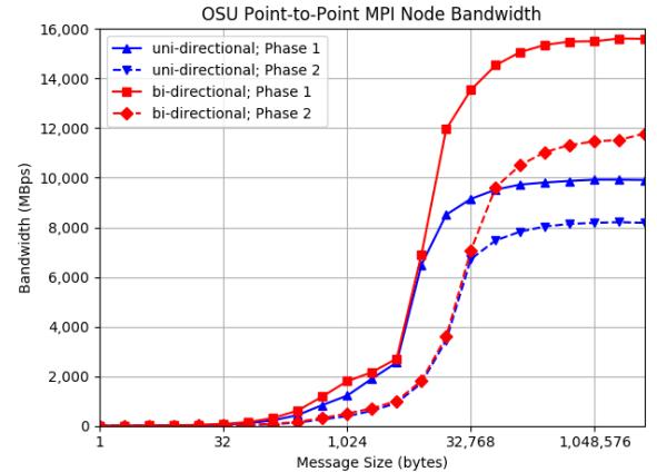
Figure 8. OMB node-to-node MPI bandwidth.
