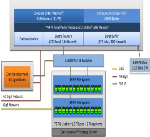
Figure 1. High-level diagram of Trinity's architecture.
