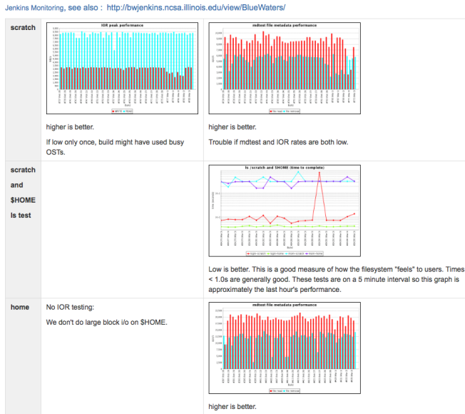
Figure 9: filesystem dashboard displaying multiple Jenkins plots
