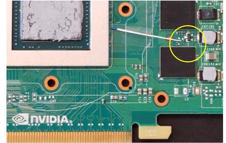
NVIDIA SXM – Location of a non-ASR that could fail prematurely due to impacts of corrosive elements
