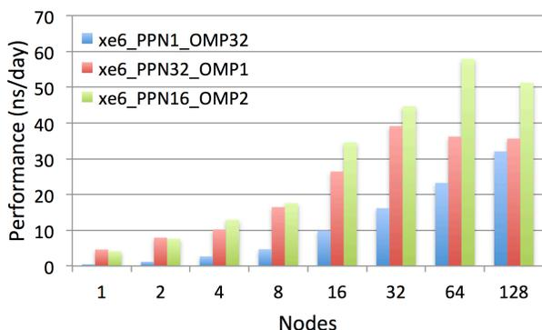
**Figure 9. LAMMPS Performance (Cray XK7)**
