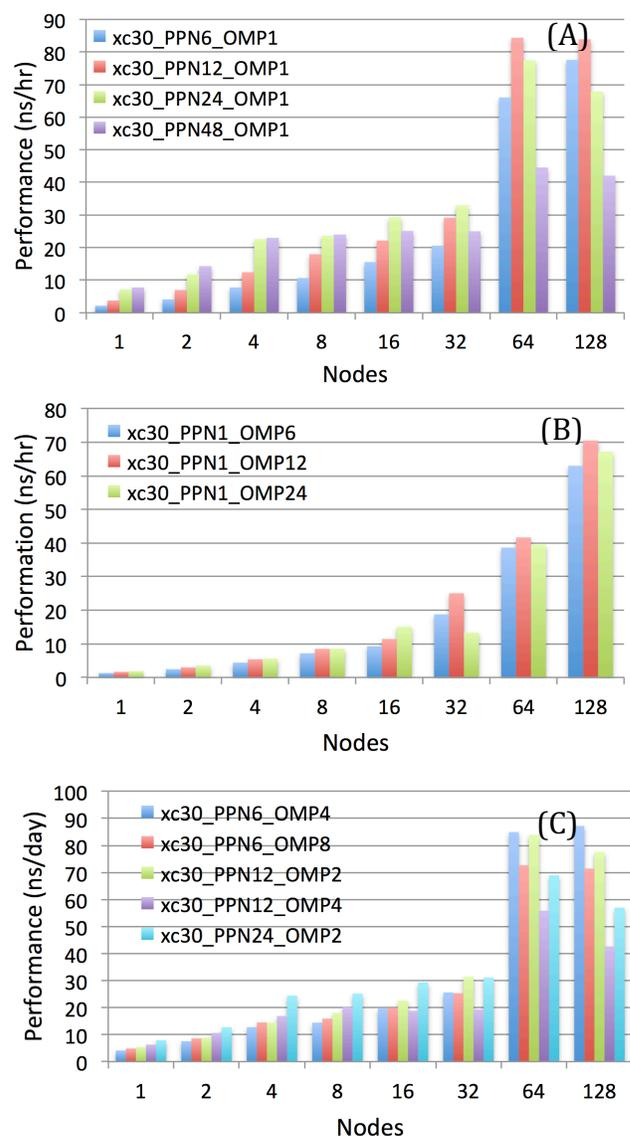
**Figure 8. LAMMPS Performance (Cray XE6)**
