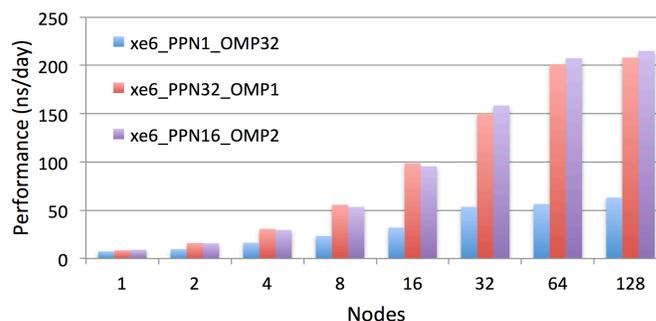
On BigRed2 XK7 nodes, the compute mode of the Tesla K20 GPUs is set as Exclusive Processing, so multiple MPI accesses to single GPU context are not allowed. Shown in Figure 6(A), when running on a small number of nodes (less than 16), jobs have better performance with more OpenMP threads. However, when the node number is large, too many threads slow down the performance.
