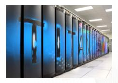
**Titan** Cray XK7 18,688 compute nodes: 1 16-core AMD Interlagos CPU, 1 NVIDIA K20X GPU Gemini interconnect
