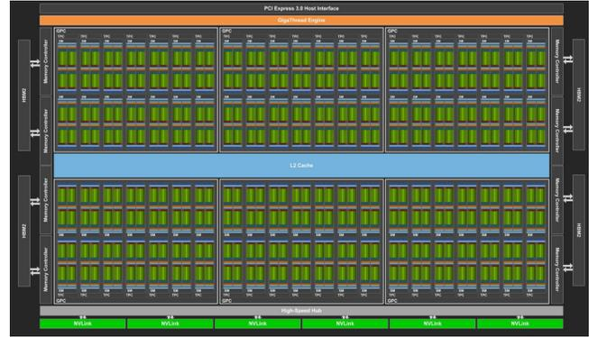
Fig. 5: Nvidia V100 GPU [1]
