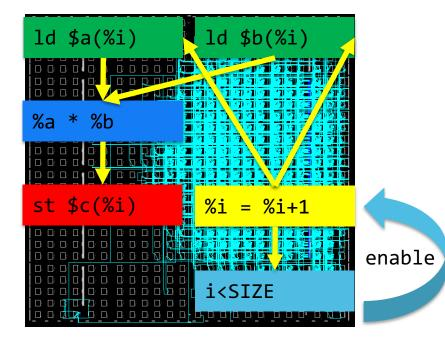
Execution on FPGA: spatial mapping of data-path and control (computing in space)
