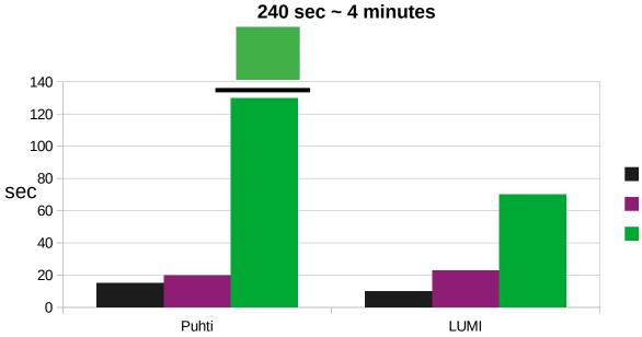
Puhti: 8 OSS 4.8PB, 57% used 484.8M Inodes used LUMI (one filesystem): 17 OSS 20PB, 9% used 45.9M Inodes used
