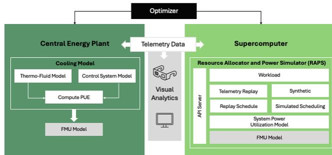
Fig. 1. ExaDigiT Facility Digital Twin (FDT) architecture [19].
