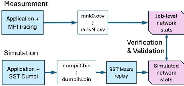
Fig. 4. Workflow for validation of network simulations.
